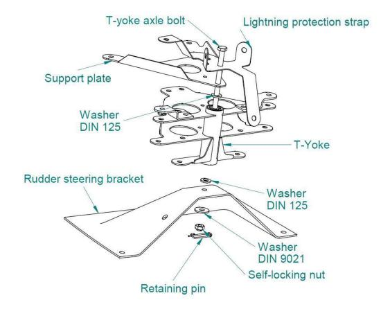
Rudder steering assembly: T-yoke and rudder steering bracket.
