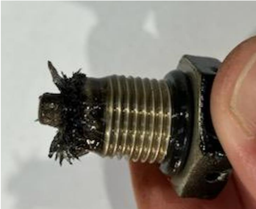
Figure 1 - Magnetic chip detector from damaged TRG.
