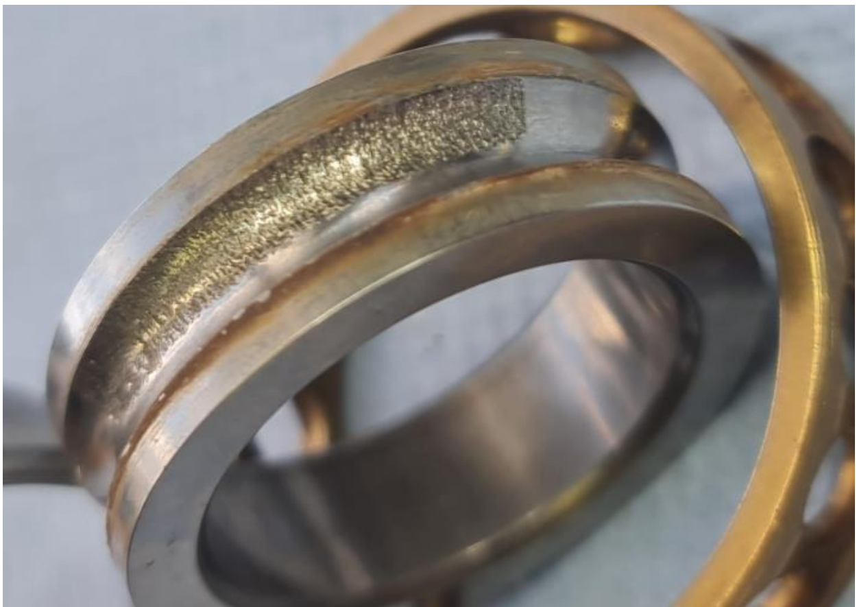
Figure 2 - Damaged duplex bearing.
