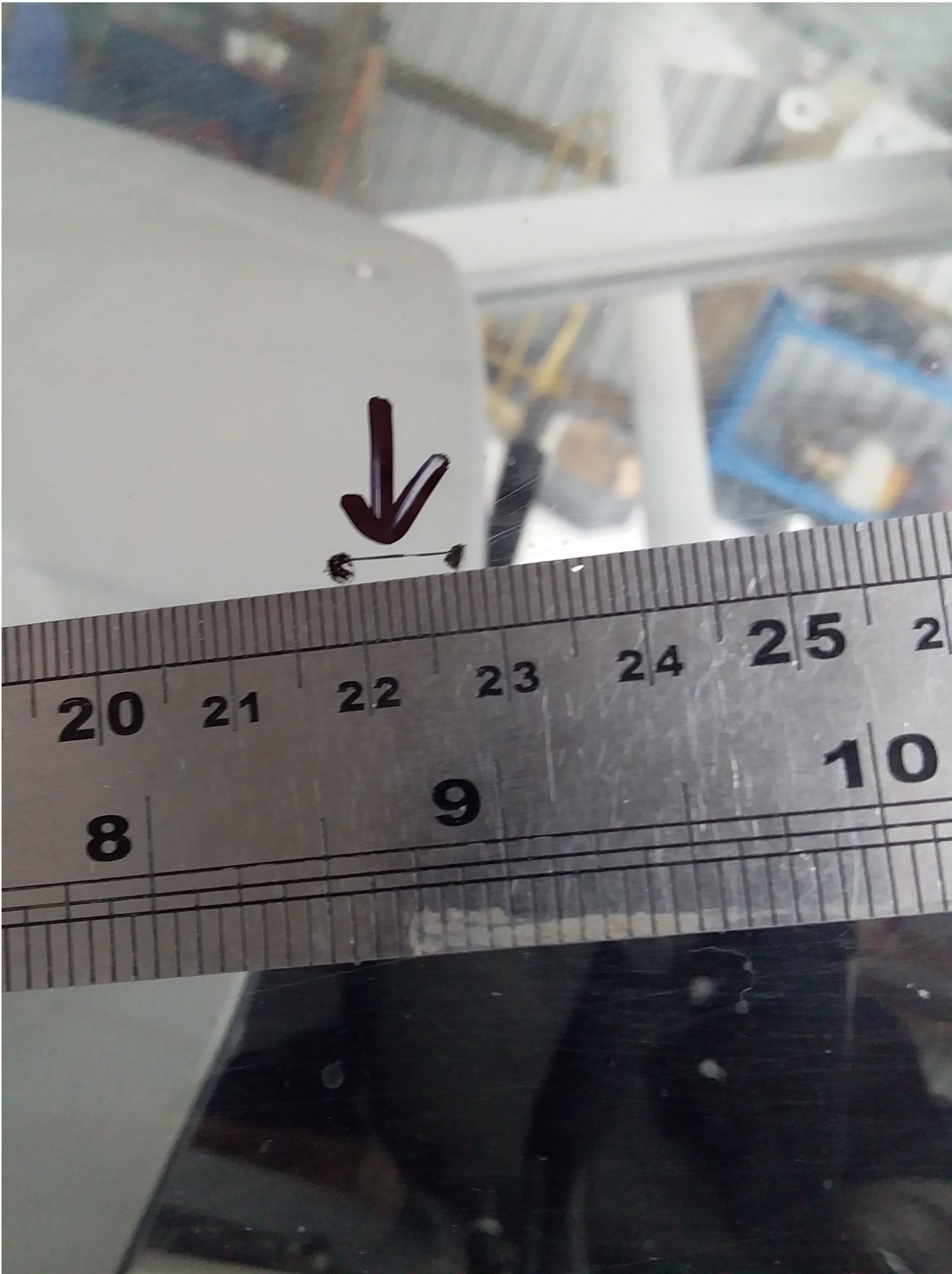
Photo 2: Windscreen LH side – Closeup of upper crack found in the A-32 windscreen. (The location of the small crack is between the dots and marked with a black arrow).
