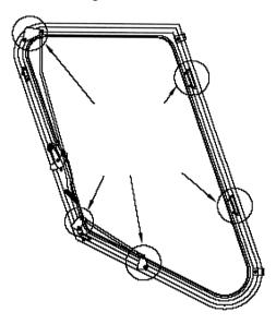
If a crack is found in any door assembly integral frame, replace LH door assembly P/N R-22-101-51 or P/N R-22- 101-53, and R/H door assembly P/N R-22-101-52 or P/N R-22- 101-54, per Tech-Tool Plastics, Inc. Installation Instructions TTP-1R, Revision A, and per the sections titled "Door Weather Seal Installation" and "Cotter Pin Installation" in Tech-Tool Plastics, Inc. Service Bulletin TTP2005-01, Revision A, prior to further flight.
