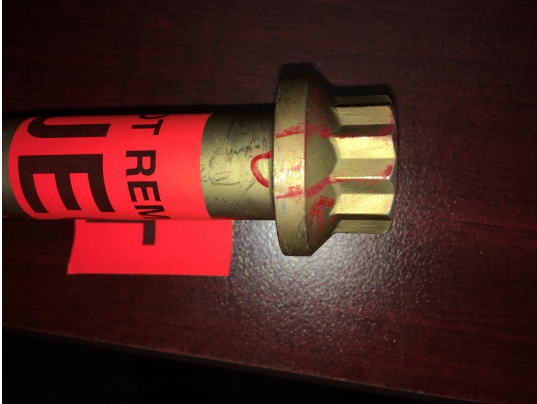
Figure 1. MS21250-12032 bolt showing area where crack was found
