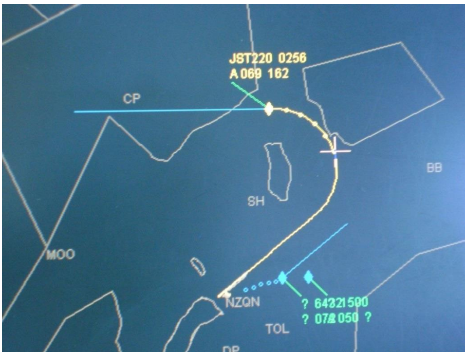
Figure 9 - Photo of Skyline information showing the level of Jetstar220 on departure. The yellow datablock JST220 has the mode C altitude information – first figures on second line (A045).
