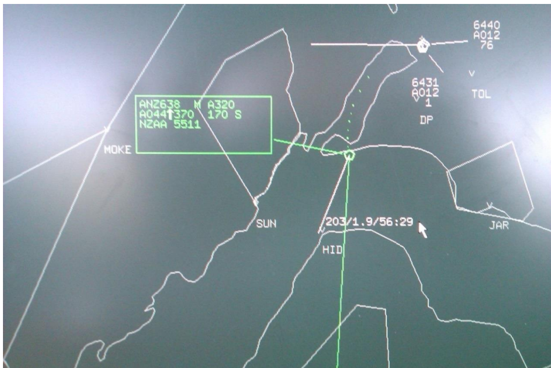
Figure 4 – Photo of Skyline information showing the level of the jet near the end of the Frankton Arm. The green datablock has the mode C altitude information – first figures on second line (A044)
