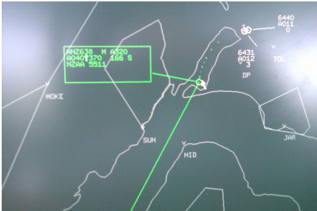
Figure 3 – Photo of Skyline information showing the level of the jet near the end of the Frankton Arm. The green datablock has the mode C altitude information – first figures on second line (A040)
