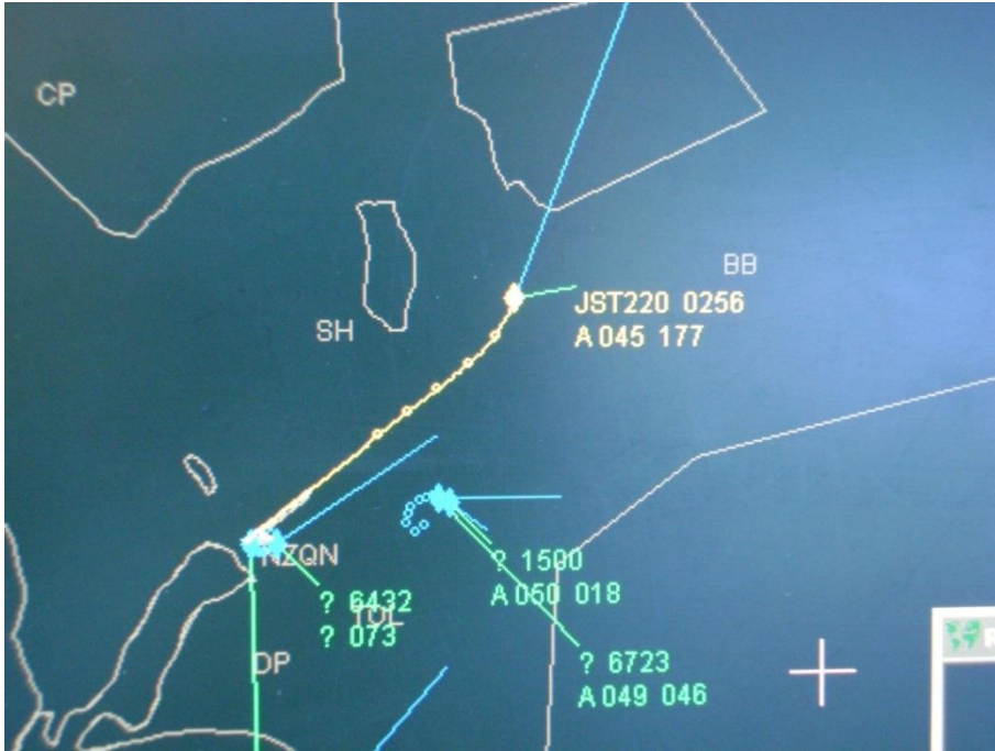
Figure 9 - Photo of Skyline information showing the level of Jetstar220 on departure. The yellow datablock JST220 has the mode C altitude information – first figures on second line (A045).
