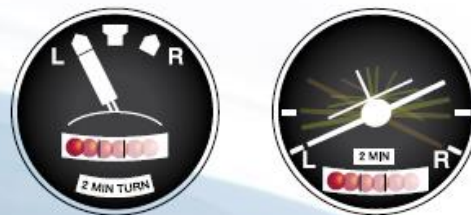
In an inverted spin, only the turn needle (left) can be trusted to show the spin direction. The ball, and the turn coordinator (right) may give unreliable readings.
