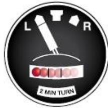
In IMC, rely on the turn needle to show direction of spin.
