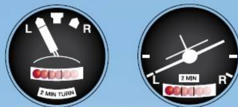
In an upright spin, both the turn needle and the turn coordinator will correctly indicate the direction of spin. The ball cannot be trusted.
