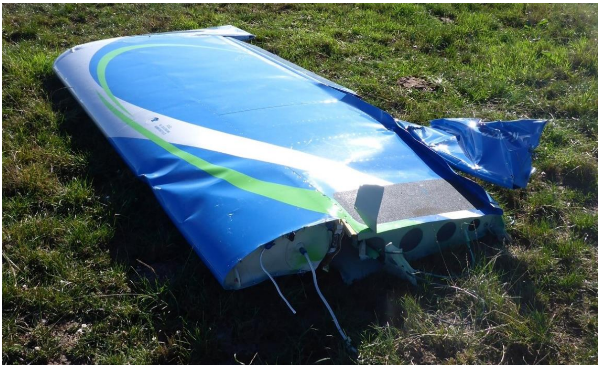
Figure 3: Right wing (Source: scene investigation)
