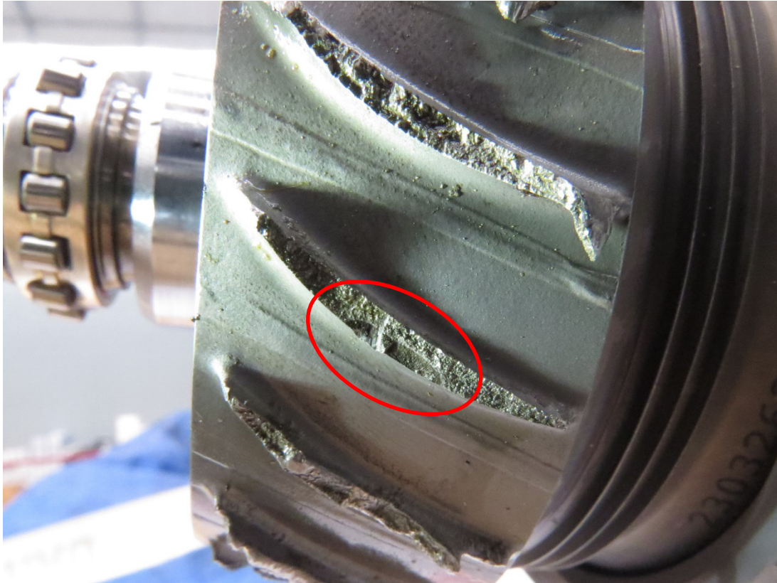
Figure 2: ZK-HQP high cycle fatigue crack in first stage blade.
