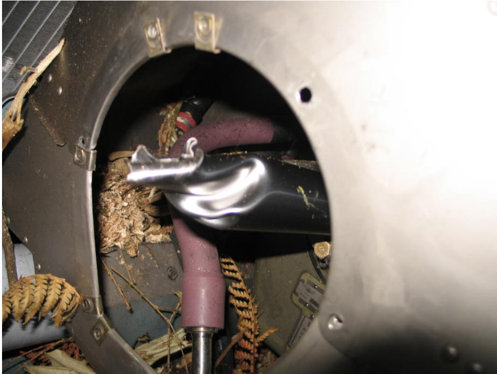
Figure 3 Torsional twisting of drive shaft.
