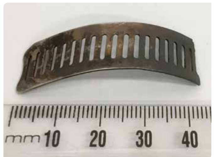
This hose clamp was found lodged in a carburettor throat, giving new meaning to the words, 'fuel contamination'.
