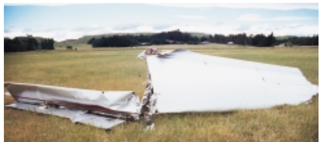
The remains of a L-13 Blanik glider wing after it suffered a complete in-flight break-up at 1000 feet. Over stressing prior to the event was thought to be a contributing factor.
