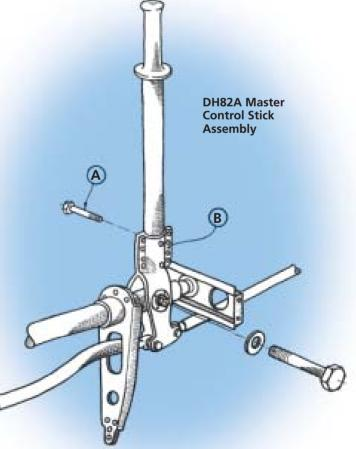
Item 'A' - The missing through-bolt on master control stick. Item 'B' – The clamping collar.
