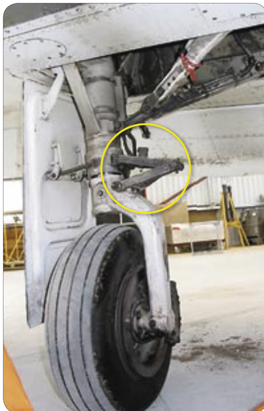
Landing gear extended – flat oleo strut. NB scissor link circled.
