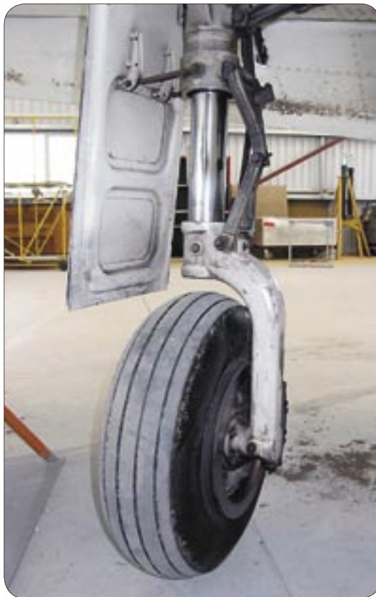
Landing gear extended – oleo strut inflated.
