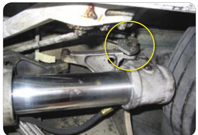
Landing gear retracted showing the up-lock hook holding the gear leg up.
