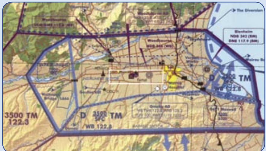
When flying in the white boxed area, when the Tower is off watch, be aware of arriving or departing aircraft at Woodbourne. Monitor 122.8 MHz.
