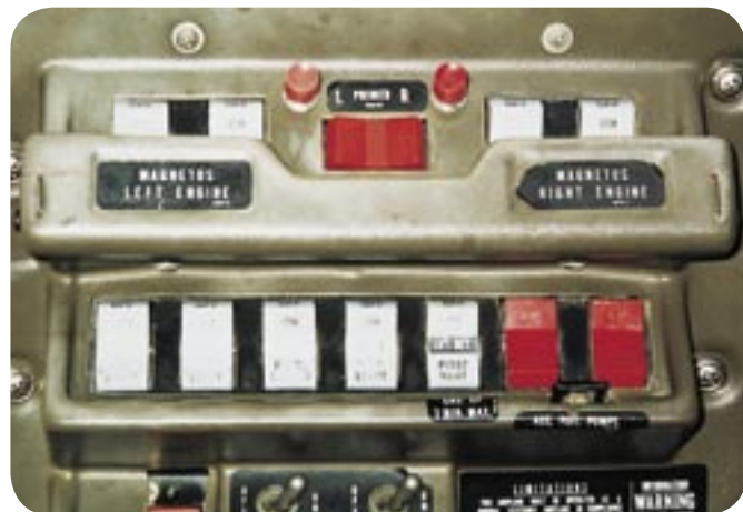
Electric priming system, on a Piper Seneca (buttons top middle).
