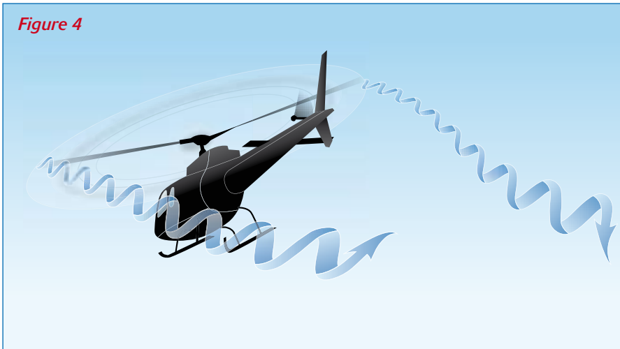
Simplified wake vortices generated from a helicopter in forward flight.
