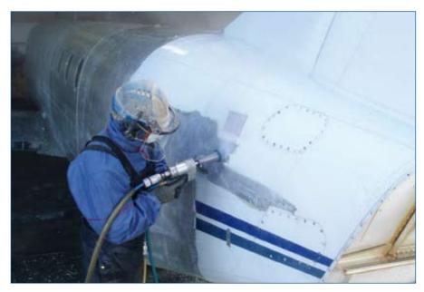
Hydroblasting uses ultra-high pressure water to remove paint.
