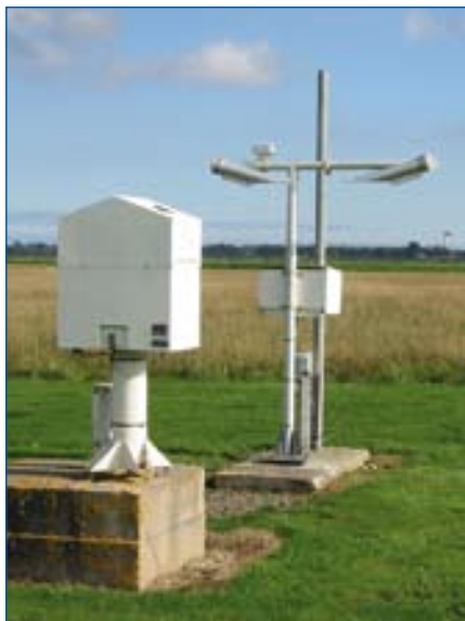
Ceilometer and present weather sensor at Invercargill.
