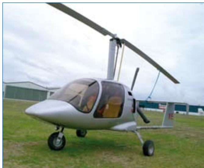
The Xenon autogyro has a fully enclosed cockpit.
