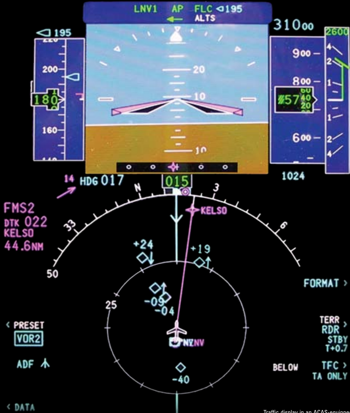
Traffic display in an ACAS-equipped aircraft. The traffic labelled +24 with a down arrow is 2400 feet above the ACAS-equipped aircraft and descending. The traffic labelled -09 with an up arrow is 900 feet below and climbing.
