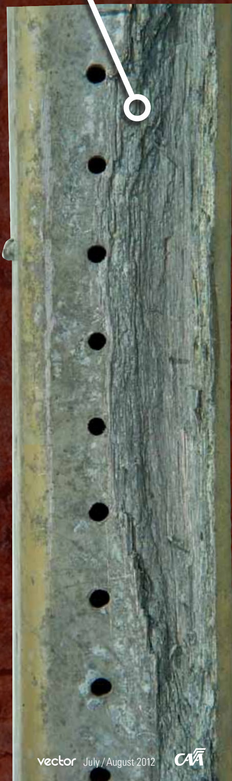
Right: An example of significant corrosion damage found in an aircraft main wing spar structural component.
