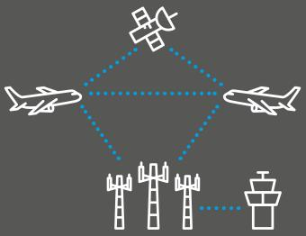
An on-board transponder broadcasts an aircraft's position, altitude, and velocity directly to air traffic control. Richer and more accurate information than that from current transponder systems means more efficient traffic management and improved safety.
