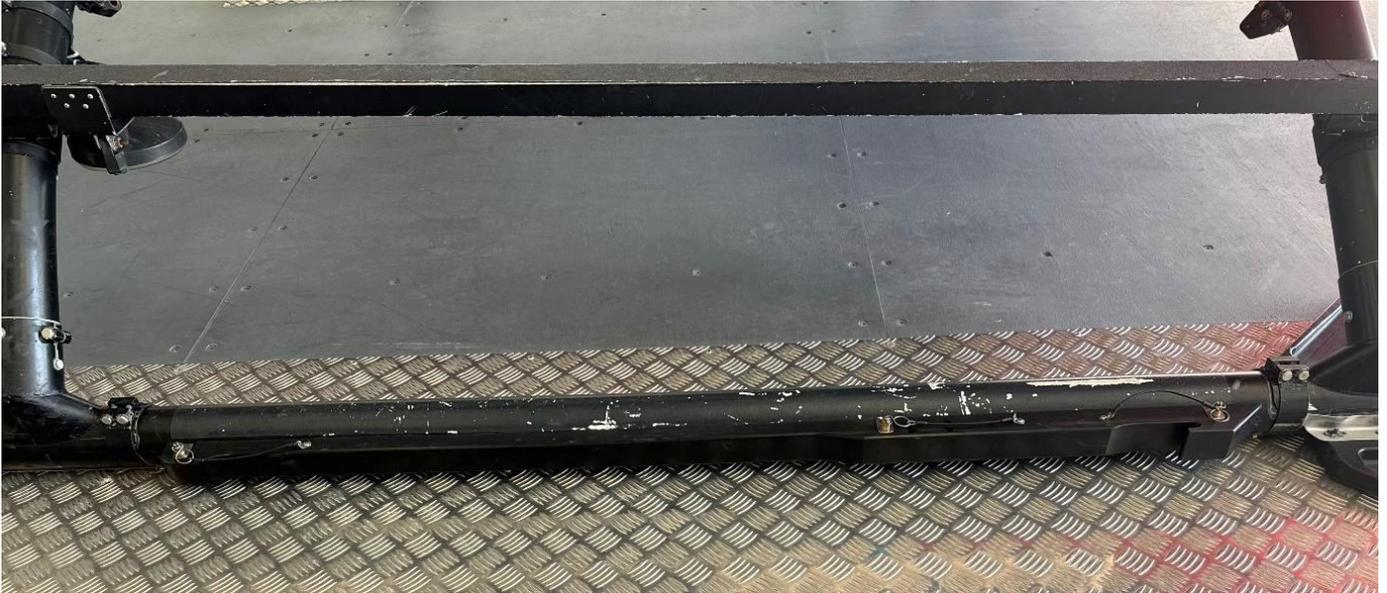
**Figure 4 - Full length cable protector installed on skid.**
