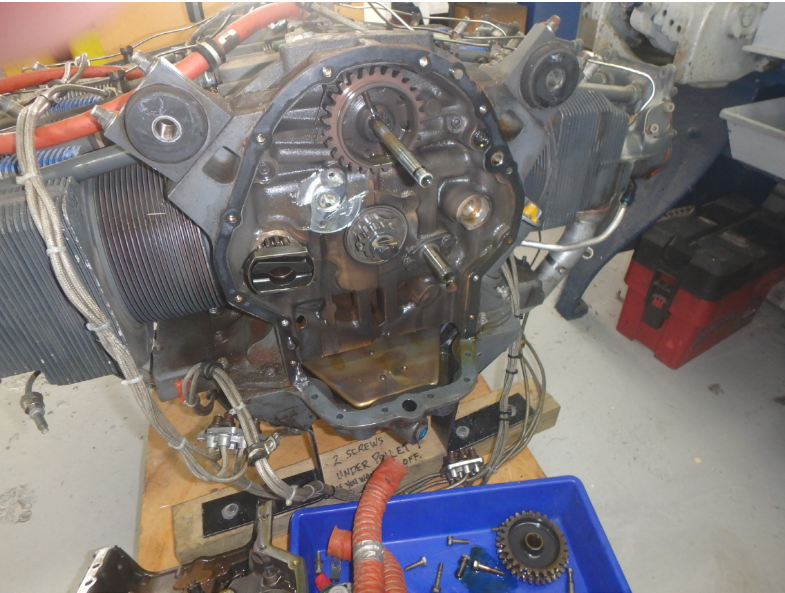
Failure of LH idler gear resulted in loss of LH magneto and camshaft drive.
